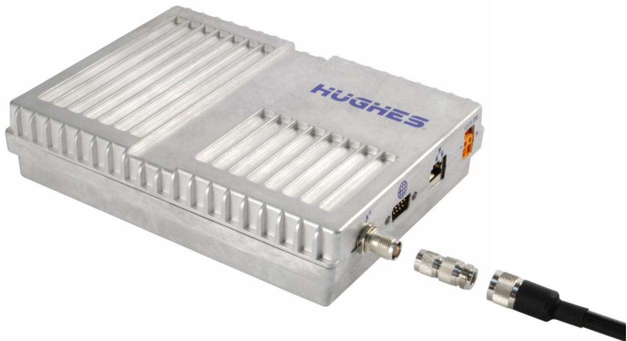
Figure 4-7 – Connect cable to TNC connector on IDU
