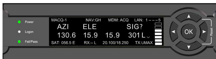
Figure 5-17: Display, confirm manual pointing direction
