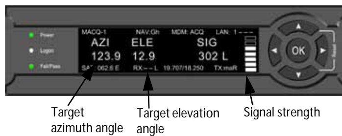
Figure 2-4: Electronically assisted tool for manual-pointing
