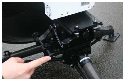
Figure 3-13: Turning the knob for azimuth adjustment
