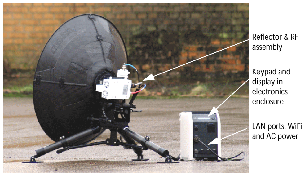
Figure 2-1: Major system components
