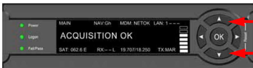
Figure 5-2: To reset the system
