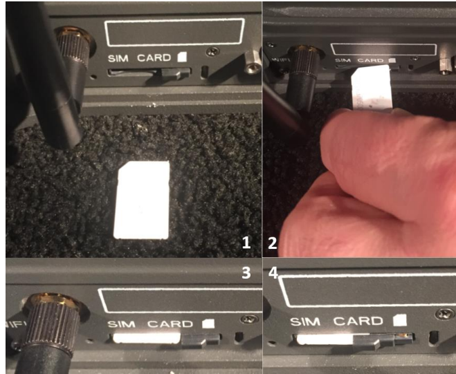
Figure 2-7 Installing SIM Card and Engaging the Lock
