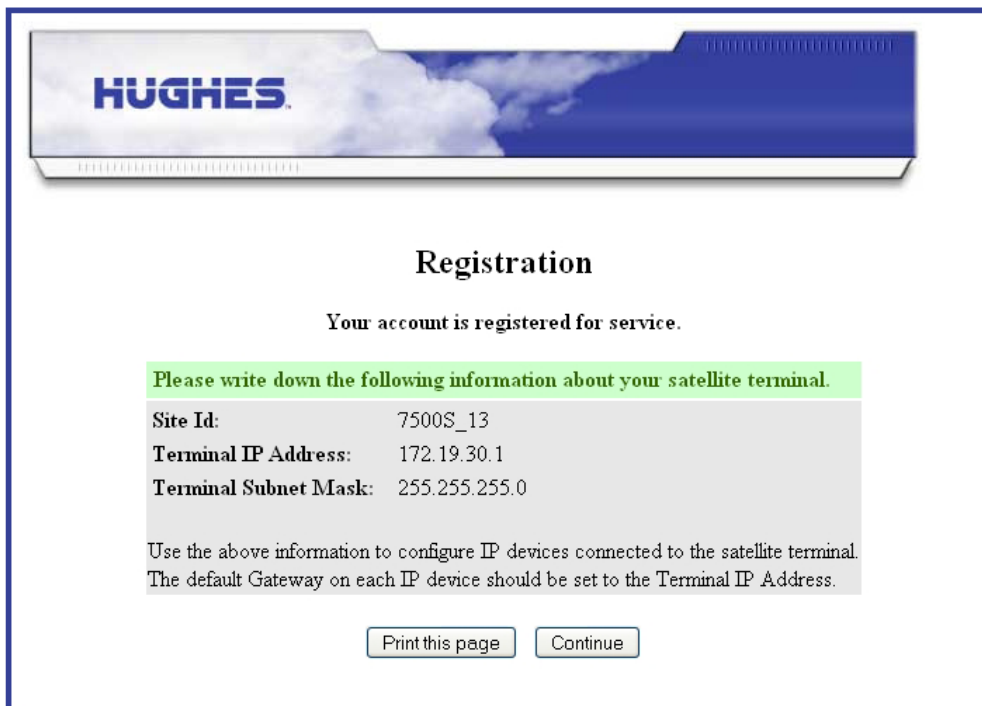
Figure 42: Registration screen with router identification information
