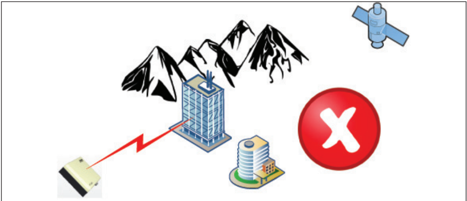
Figure 2: Poor Terminal Location - Line of Sight Blocked by Obstruction
