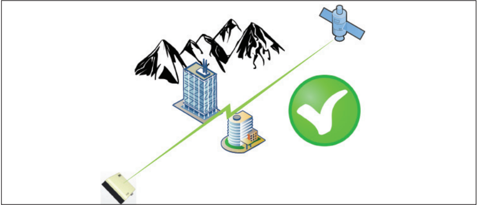
Figure 3: Good Terminal Location - Line of Sight Clear
