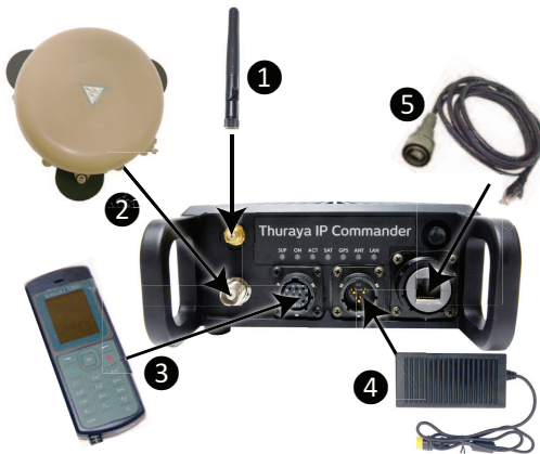
Figure 3: Hook-up Diagram (numbering same as above)
